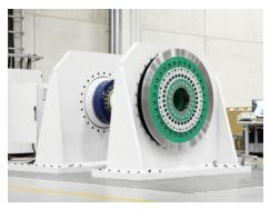
Initial testing sample on the new test bench is a torque limiter having set a torque of more than 350,000 Nm
